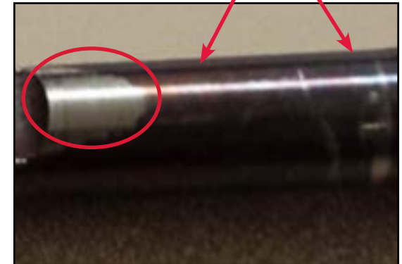
Wear area (circled) of chain pin after six weeks with Chesterton 690 FG Lubricant .
